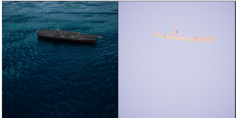
Fig. 4 Example surface normal map generated with LookSIM; normal vectors are color-coded
